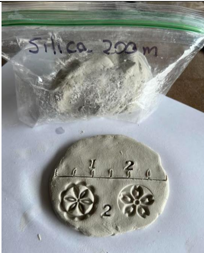
Shrinkage test tile.
